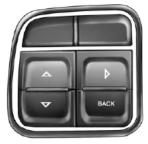
Press the button to view a graphic of the vehicle with a tire pressure value at each corner of the graphic.
