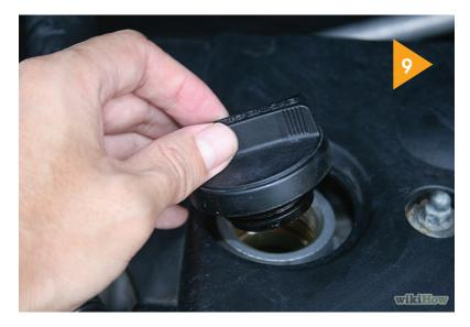
**Note:** You do **not** add oil into the tiny tube that the dipstick sits in. Look for a screw-off cap on top of the largest part of the engine. It could be blank or it could be labeled "Oil Cap", and it might even indicate which grade of oil you ought to be using in your car. Unscrew that cap and add oil as needed.
