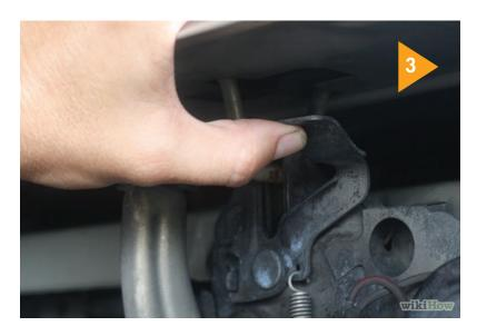
4. Prop up the hood solidly. Some hoods stay up by themselves. Most hoods have a hood prop - a long, thin metal rod attached either to the underside of the hood or to the bottom edge of the hood opening. Either lower or lift the rod (depending on where it is located) and fit the end of it into the slot that is provided to hold it in place. Make sure that the hood is secure.
