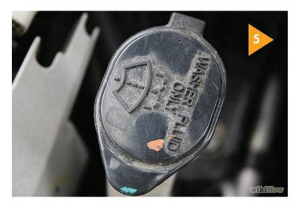
6. Check the washer fluid level. The tank is usually translucent, allowing you to see whether there is fluid in the reservoir or not. Many washer fluid reservoirs have marks to show the fluid level. If the tank is less than halffull, you will need to refill it.
